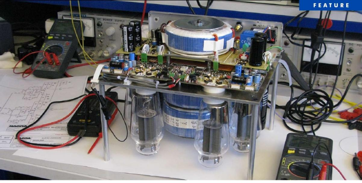
At the next workstation, we saw Nagra's latest creation, a 60-watt-per-channel solid-state amplifier that had debuted at CES this January. It was plugged into a massive test bench with every possible parameter being measured. Upside down in the same room was a working prototype of a new vacuum-tube power amplifier featuring 300B tubes.
